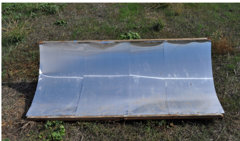
Fig. 2. Front view of concave solar concentrator.
