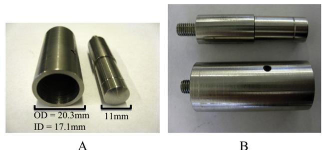
**Fig. 2.** Front (A) and side (B) views of the hollow probe (left side in A, bottom in B) and Magness–Taylor solid cylindrical probe (right side in A, top in B). The hollow probe features a 17.1 mm inner diameter and 20.3 mm outer diameter. The solid probe is 11 mm in diameter.
